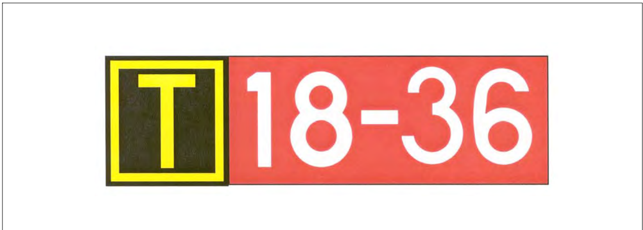
FIG 2-3-31 Taxiway Location Sign Collocated with Runway Holding Position Sign
