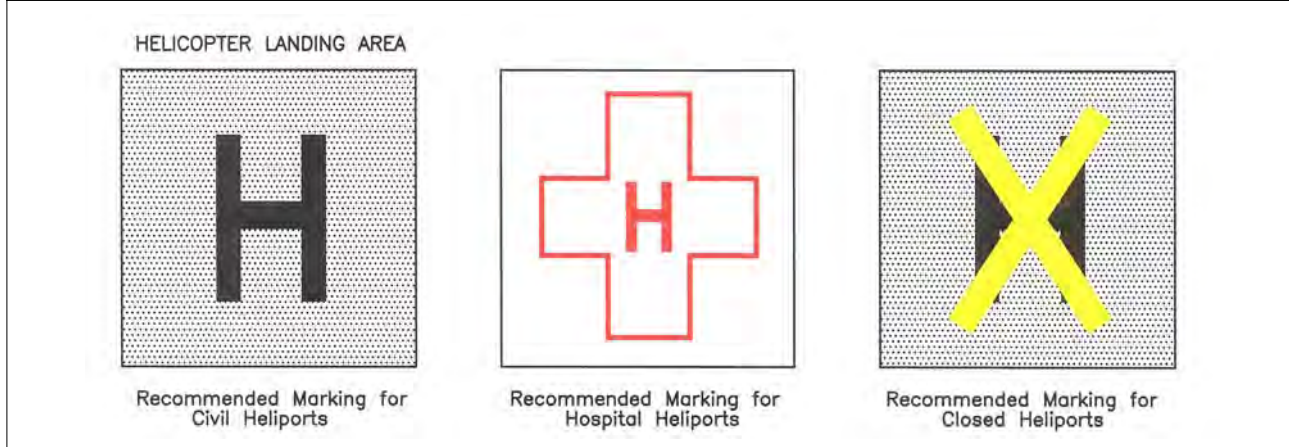
FIG 2-3-23 Helicopter Landing Areas
