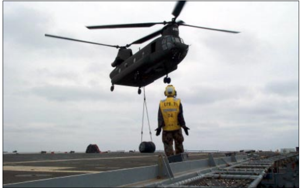
A HOOKMASTERS CH-47D slingloads a blivet onto a shipdeck during a recent training exercise.
