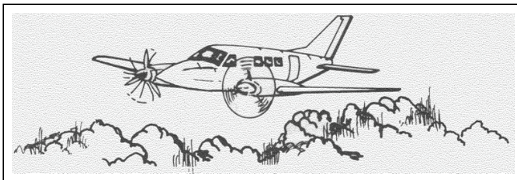
Figure 7-62. Windmilling propeller creating drag
